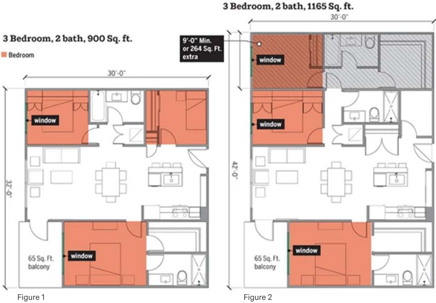
Figure 2 illustrates a 3 bedroom unit layout and size typically seen in the City of Vancouver, with all three bedrooms located against an exterior wall in order to have direct access to daylight.
