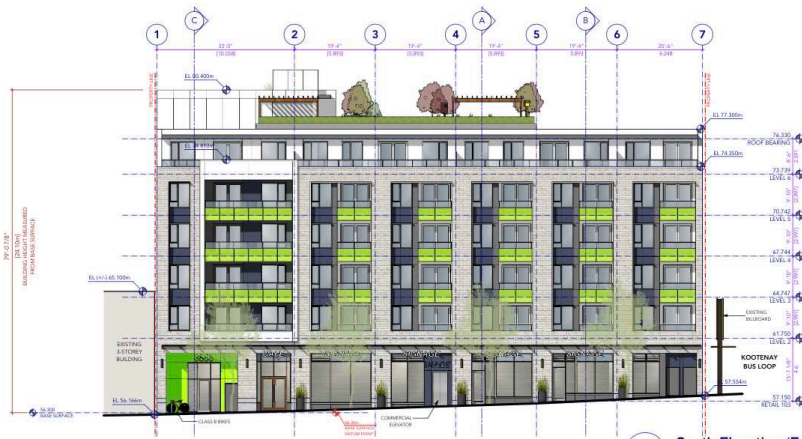
1 South Elevation (East Hastings Street) Scale: 3/32" = 1'-0"
