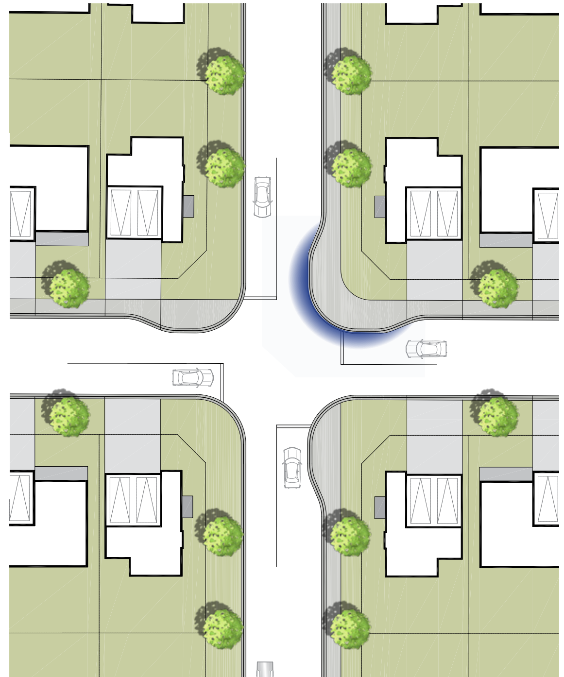
Figure 31 Double Bulb-Out at Intersection
