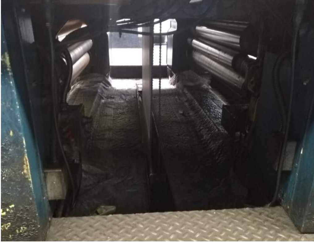
Photo 10: Adsorbent sheets and visible grease/oil on printing press
