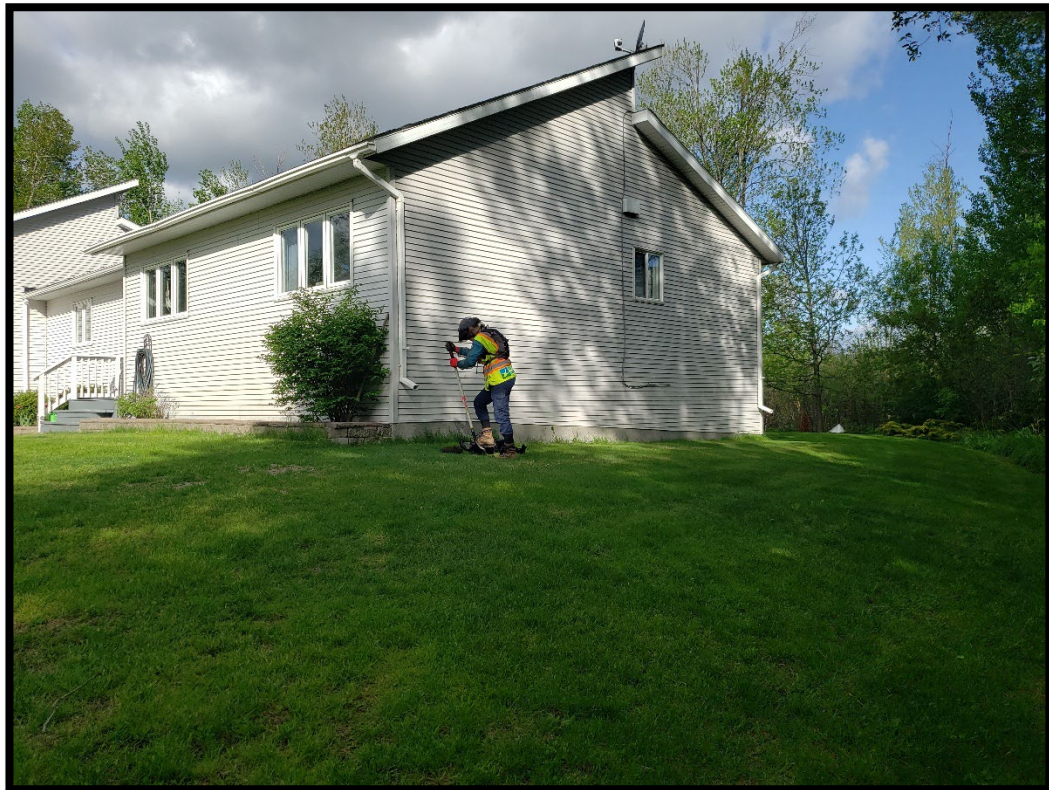
Figure 16: Test pitting in progress (MH1511-D018).
