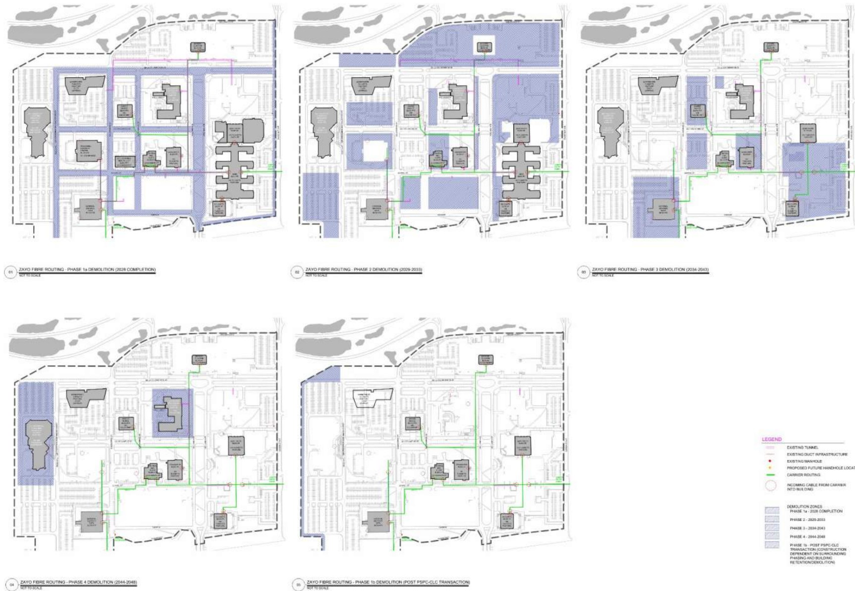
Figure 20: Zayo Fibre Routing Demolition (By Phases)
