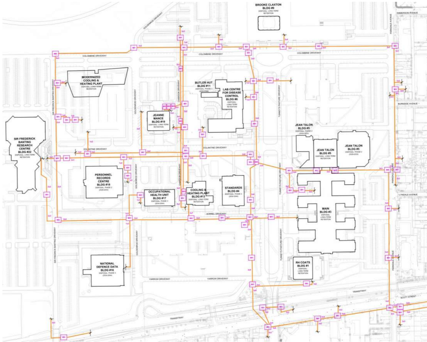
Figure C.1: Hydro Ottawa Current Duct Infrastructure Site Plan (Purple Manholes, Orange Duct Pathways) (2025-09-25) (Attain Drawing Page #8)
