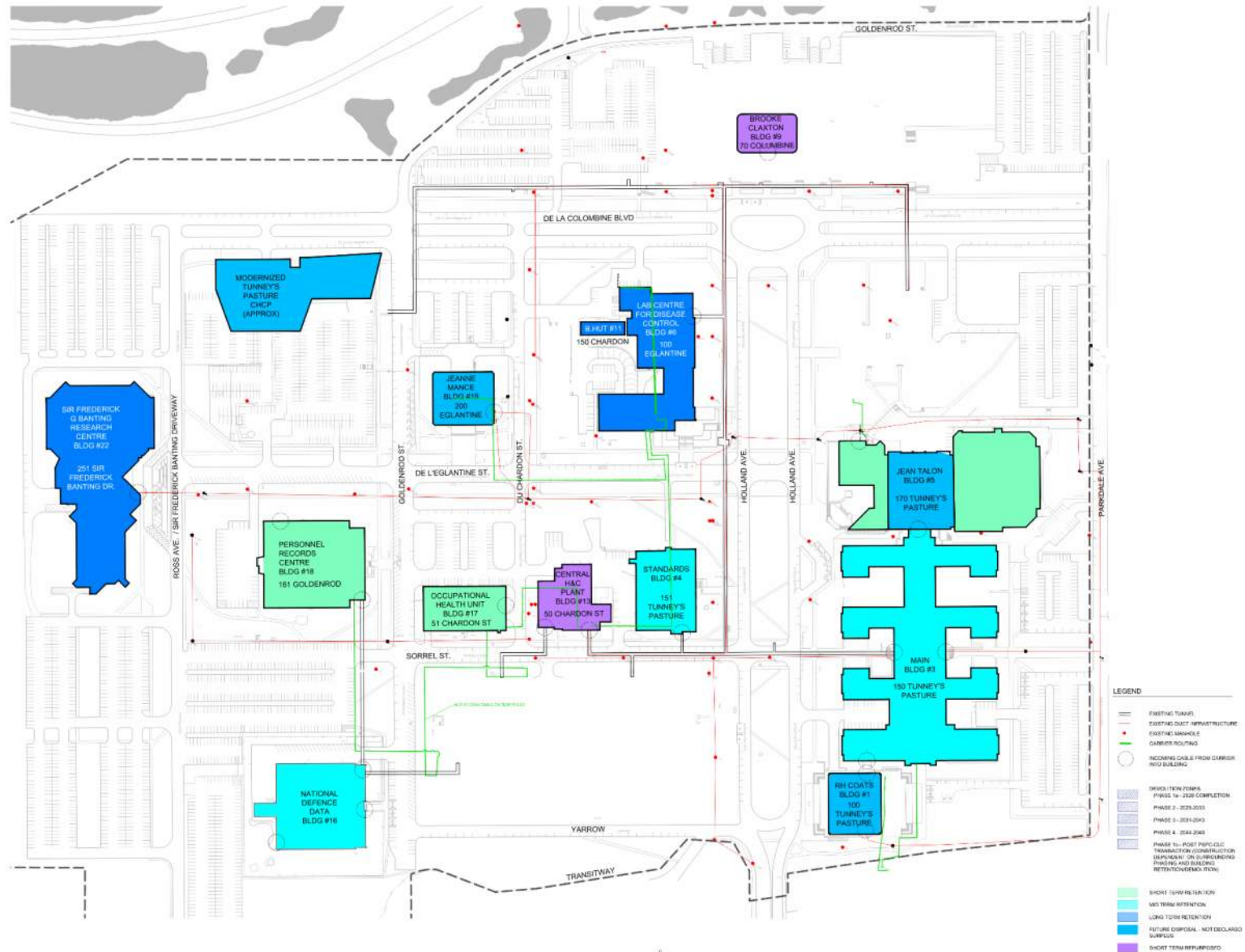
Figure 5: Existing Rogers COAX Routing at Tunney's Pasture
