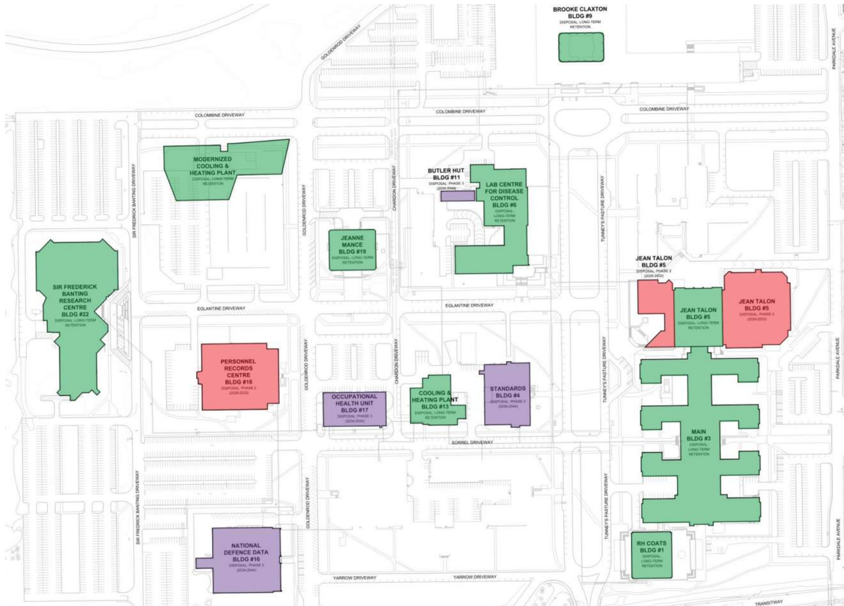
Figure 6.1: Proposed Building Phasing Plan – Phase 2 (Red), Phase 3 (Purple), Phase 4 (Green) (Attain Drawing Page #2)
