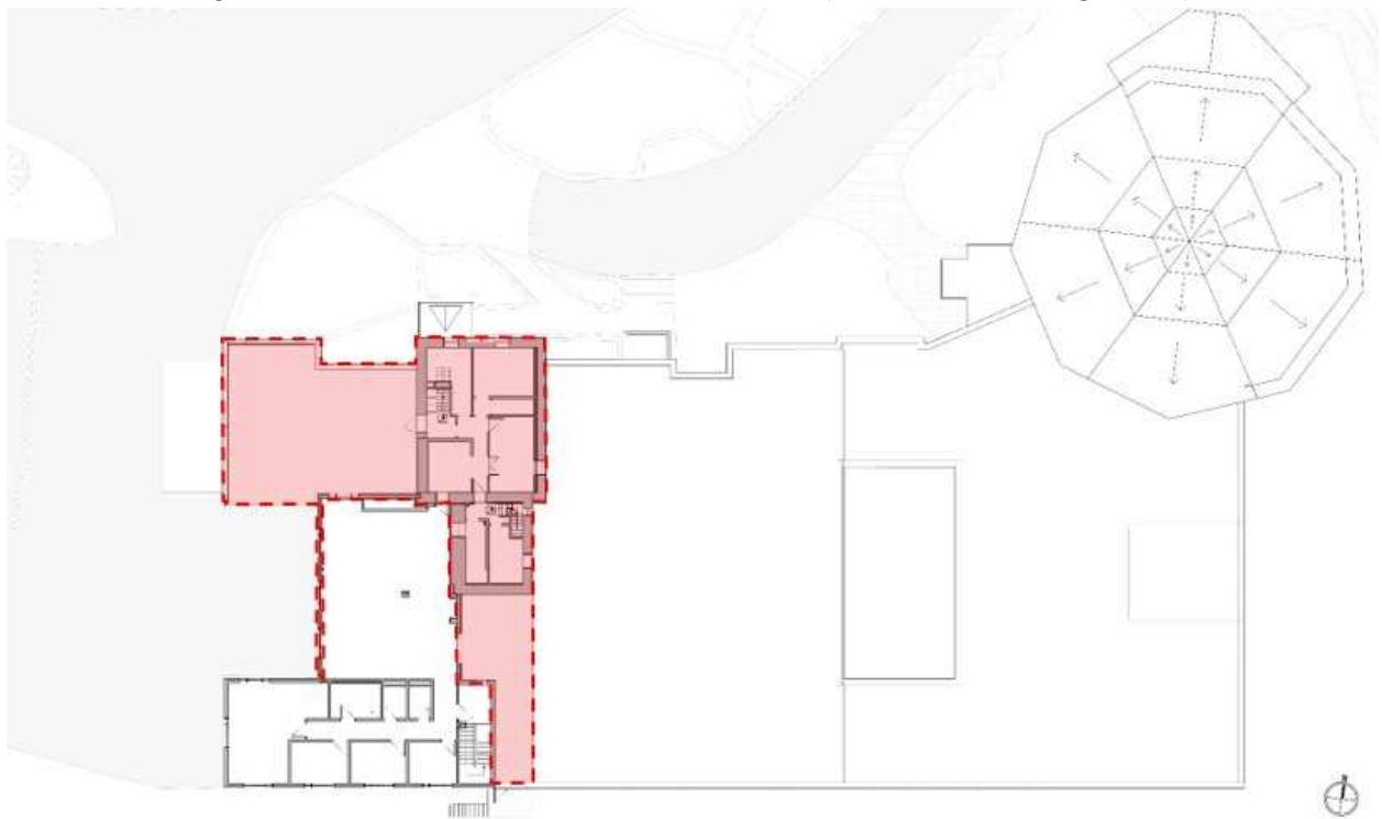
Figure 36 – 2 nd Floor demolition, all areas in red hatch (RMA+SH architects, August 2026)
