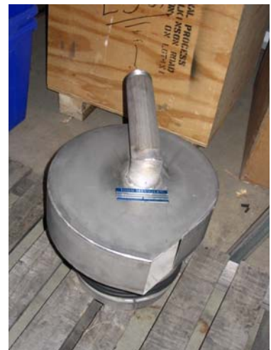
VHV with air vent for minimal slopes
