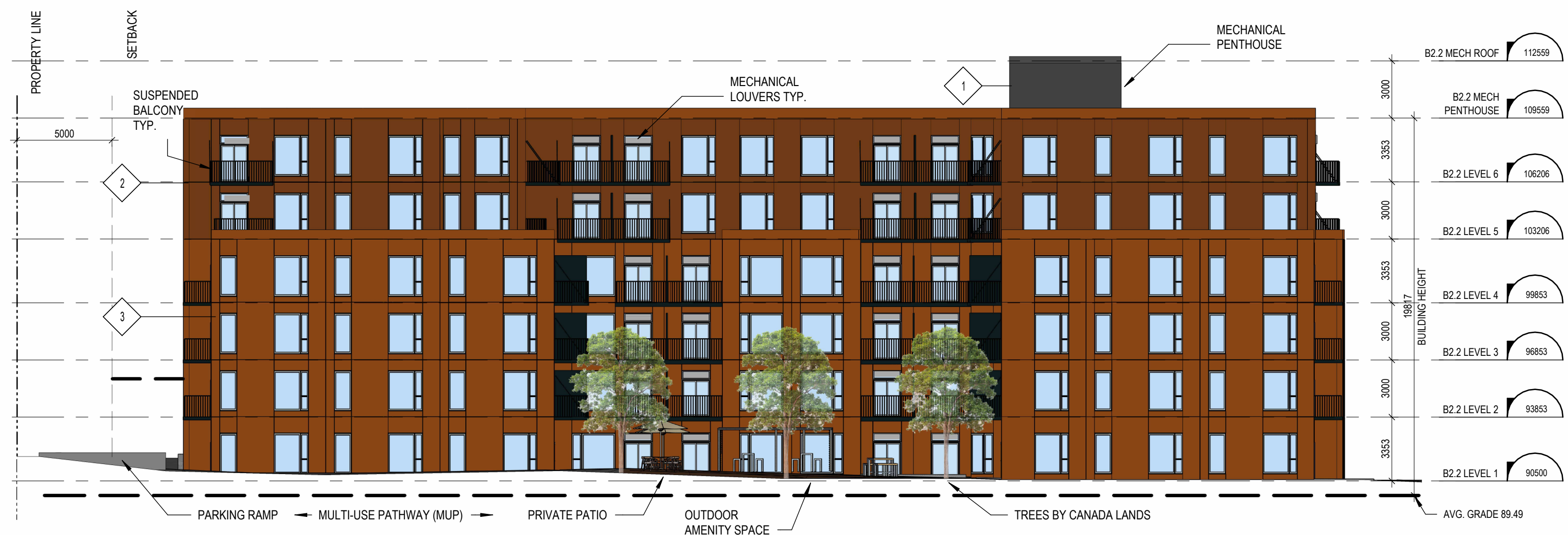
2 BUILDING B - WEST ELEVATION ÉCHELLE / SCALE: 1:200 A.201
