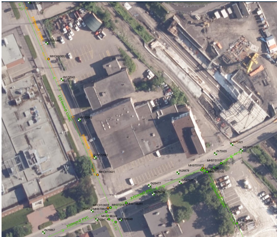
Figure 4-1 Existing Storm Sewer Services
