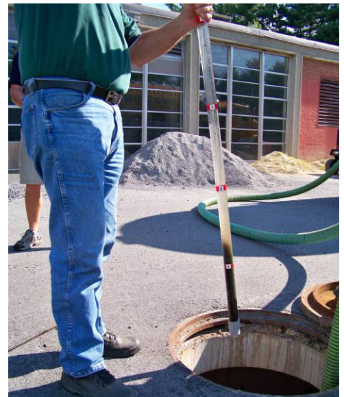
The depth of sediment and oil can be measured from the surface by using a sediment probe or dipstick tube equipped with a ball check valve and inserted through the Jellyfish Filter's maintenance access wall opening. The large opening provides convenient access for inspection and vacuum removal of water and pollutants.
