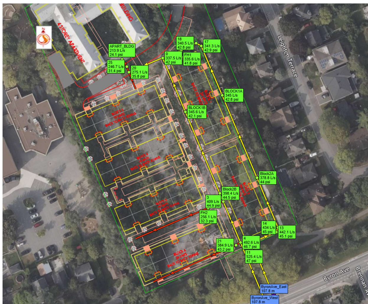
Figure 3-4: Residual Pressure (psi) for MXDY+FF (200L/s) Demands
