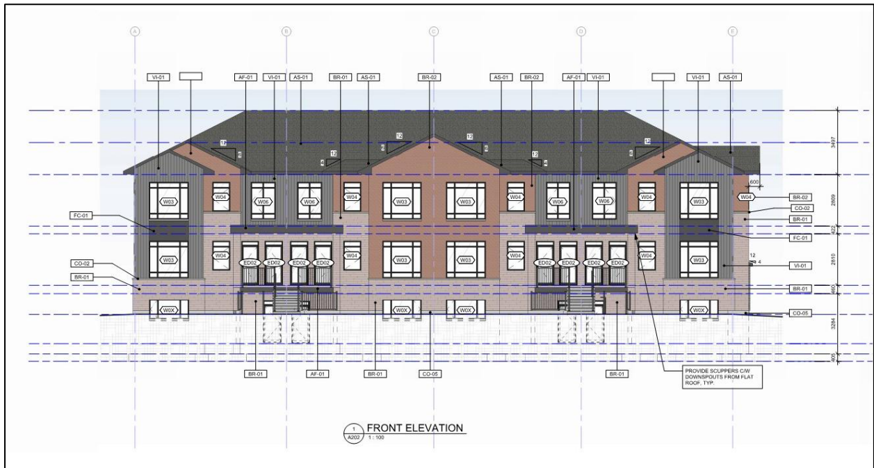
Figure 13: Front elevation of the stacked low-rise building prepared by RLA Architecture Inc.
