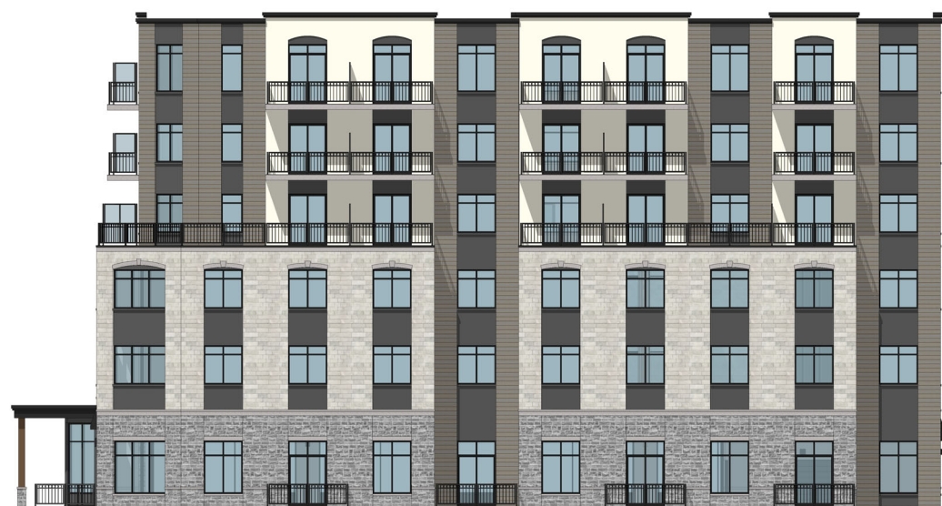
Design Evolution No. 3 – East façade of Phase 1 building viewed from Bareille-Snow Street with split lower level cladding & fenestration
