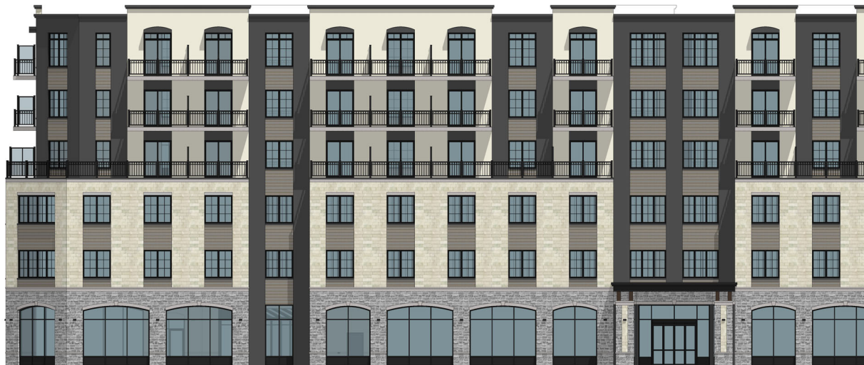
Design Evolution No. 2 – South façade of Phase 1 building viewed from Tawadina Road with ground floor arched window openings & precast stone lintels above
