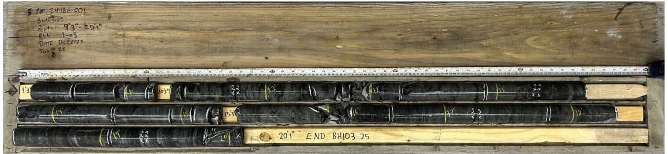
Borehole BH103-25 Rock core runs 1 through 3, 2.8 to 6.1 mbgs
