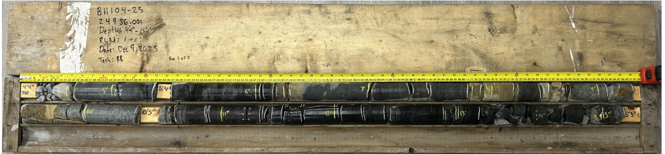
Borehole BH104-25 Rock core runs 1 through 3, 1.3 to 4.7 mbgs
