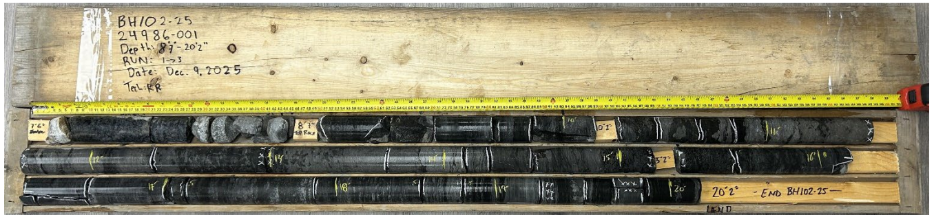
Borehole BH102-25 Rock core runs 1 through 3, 2.6 to 6.1 mbgs
