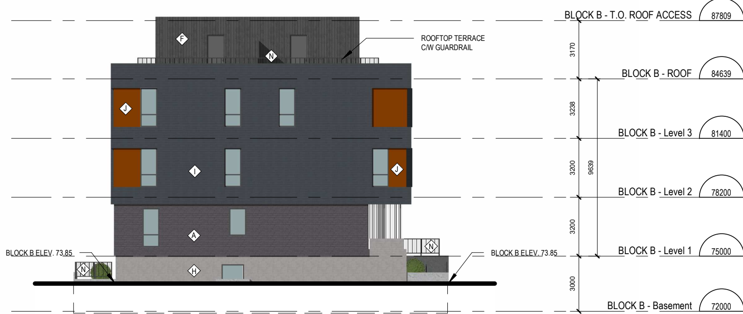
7 TOWNHOME BLOCK B - NORTH ELEVATION ÉCHELLE / SCALE: 1:200
