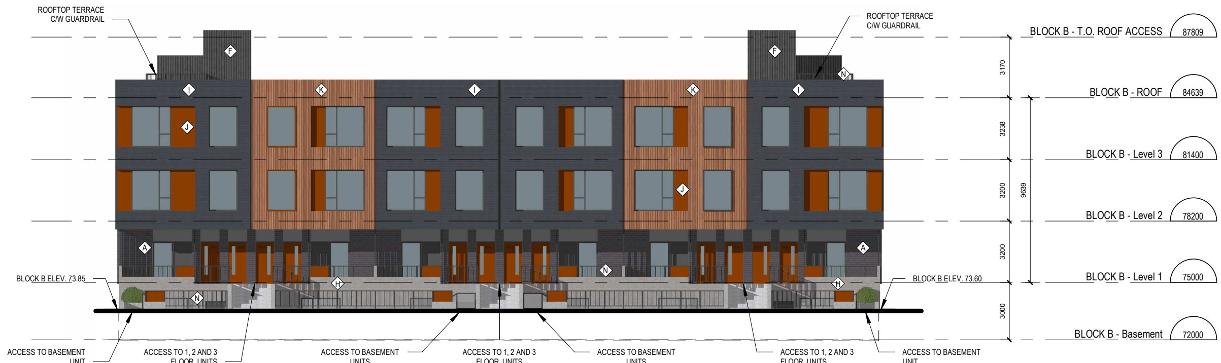
5 TOWNHOME BLOCK B - WEST ELEVATION ÉCHELLE / SCALE: 1:200
