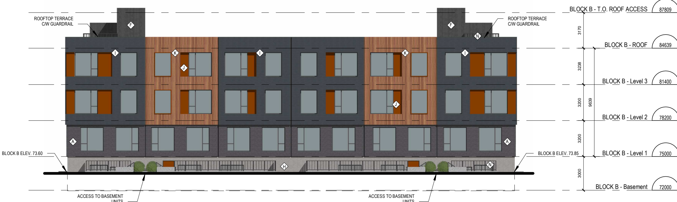
8 TOWNHOME BLOCK B - EAST ELEVATION ÉCHELLE / SCALE: 1:200
