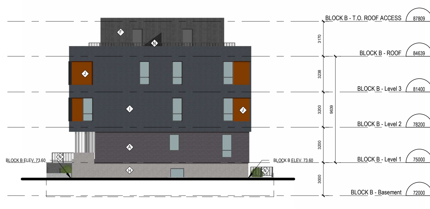
6 TOWNHOME BLOCK B - SOUTH ELEVATION ÉCHELLE / SCALE: 1:200
