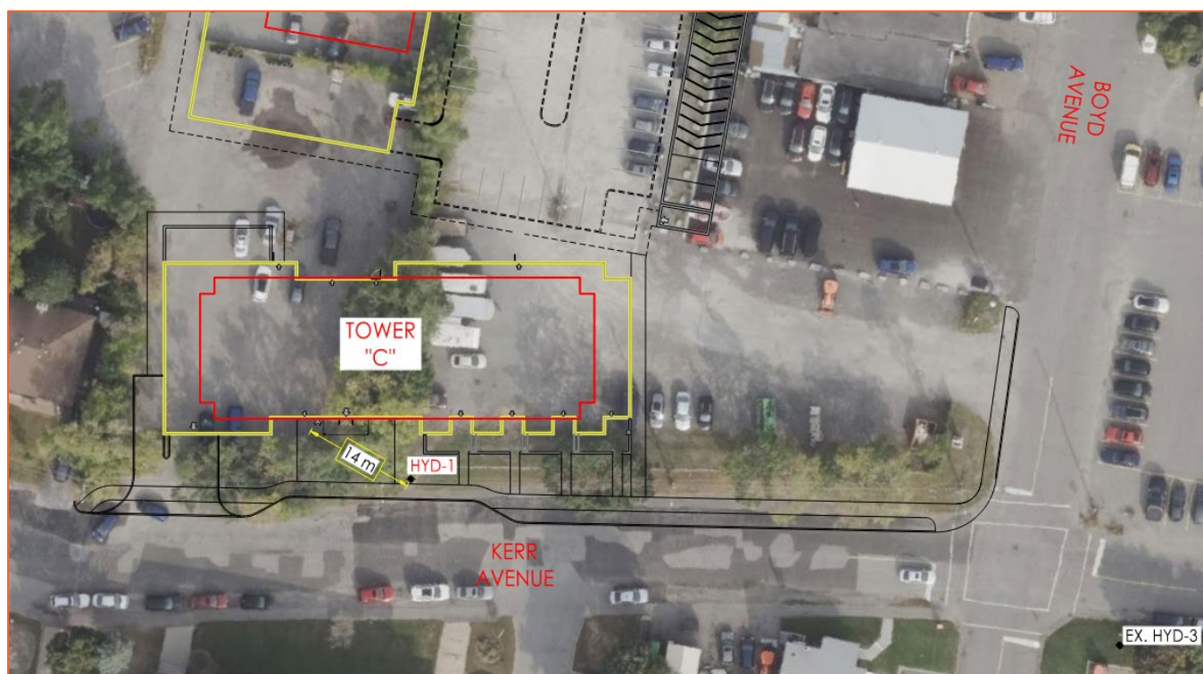
Figure 3.1: Fire Hydrant Coverage Sketch
