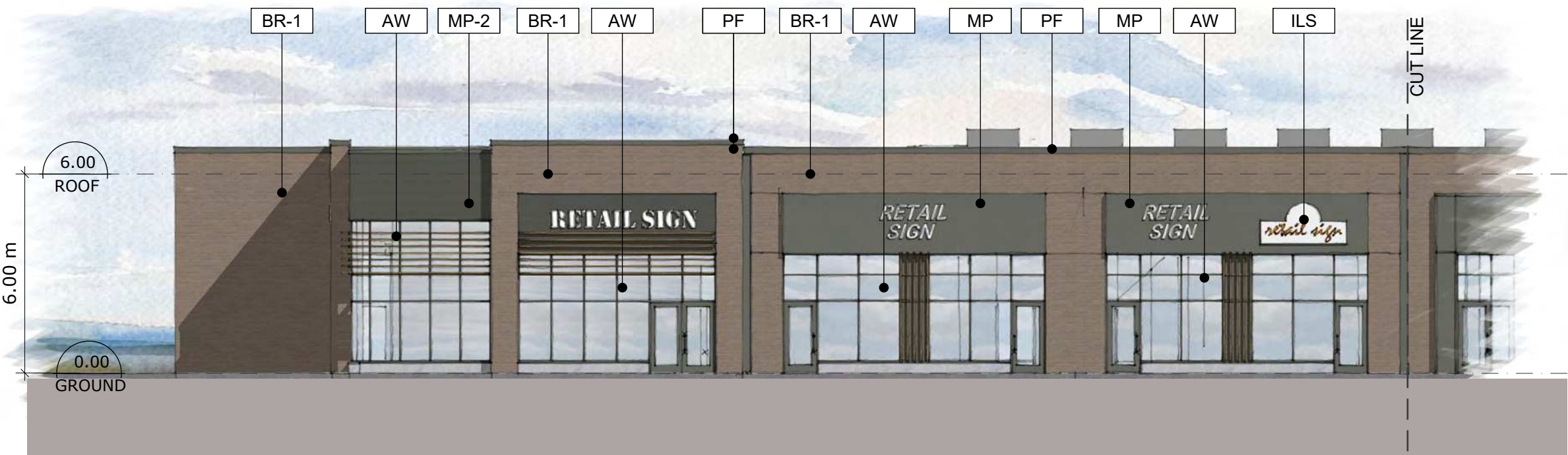
CRU 6 - SOUTH ELEVATION (WEST HALF)
