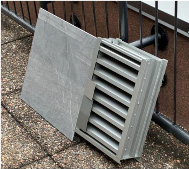
Figure 2.2-1: Photograph of Porcelain Panel with polished finish and metallic louvre sample
