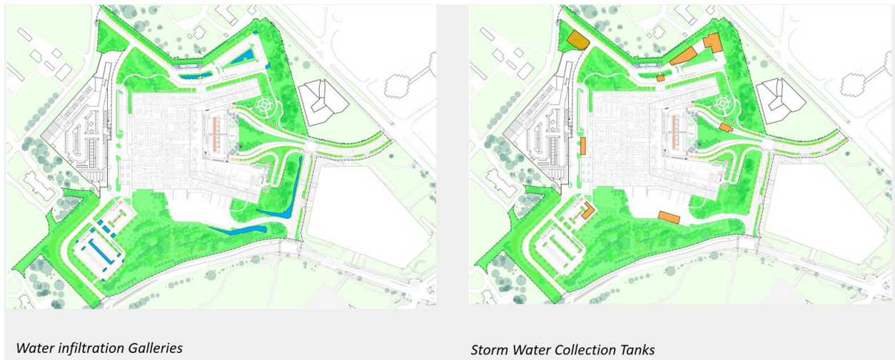
Figure 3.3-2: Infiltration areas and stormwater tanks
