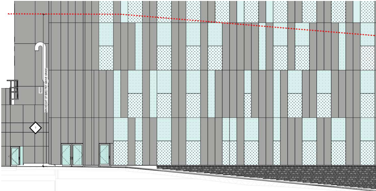
Figure 1.0-1: The Red line shows a typical identifier of 16m above grade for bird-safe treatment (Extract from elevation drawings)
