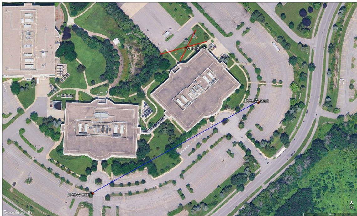
Figure 1: VES (red) Survey lines.
