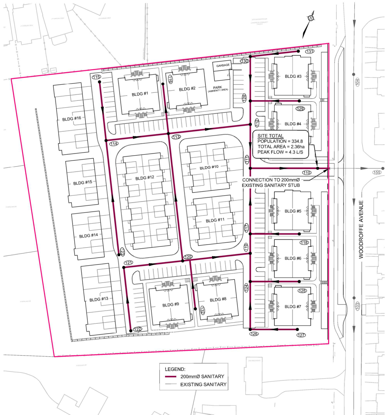
Figure 4: Sanitary Sewer Network
