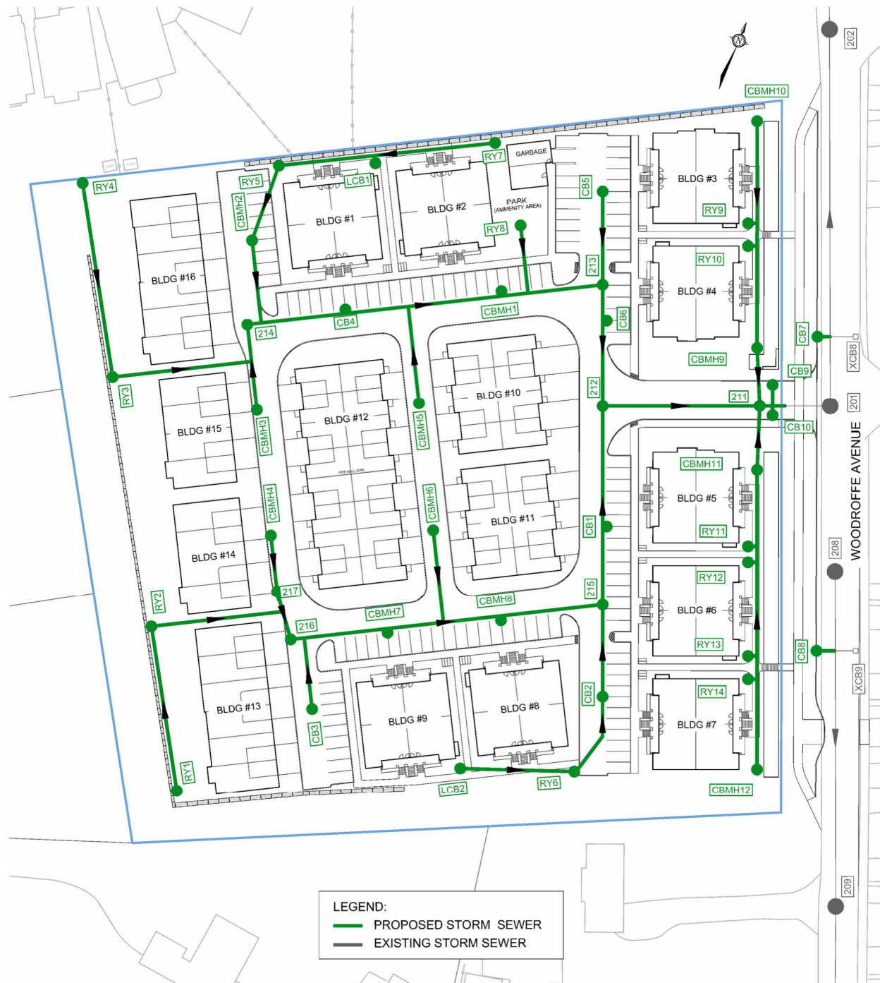
Figure 5: Storm Sewer Network
