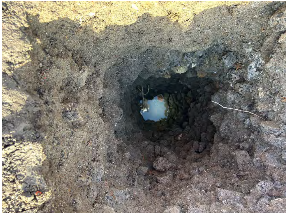
Photo 2 - View of test pit TP-02
