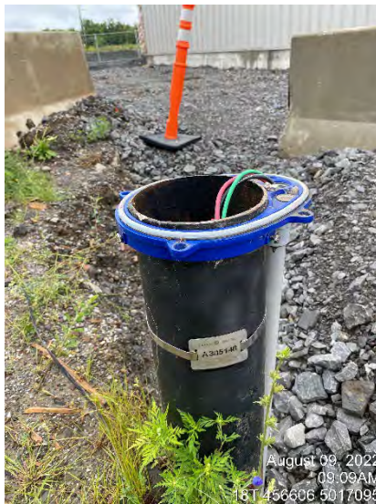
Photo 4 - Observation well (ID A305146) used during pumping test for monitoring of potential interference effects.
