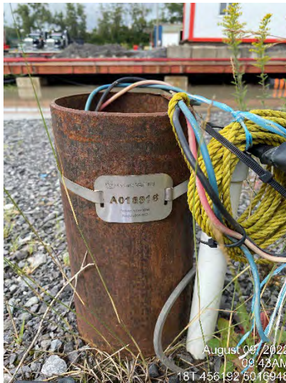
Photo 7 - Observation well (ID A018916) used during pumping test for monitoring of potential interference effects.
