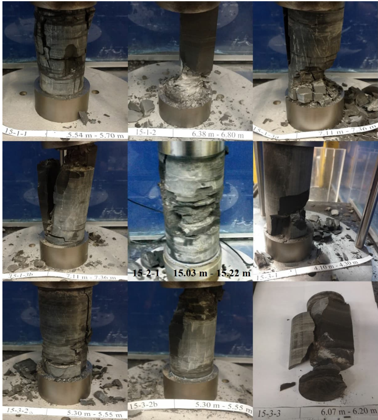
Figure 4: Photographs of UCS specimens after testing.
