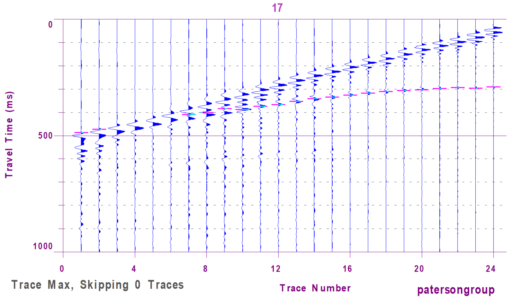
Figure 3 – Shear Wave Velocity Profile at Shot Location 73.5 m
