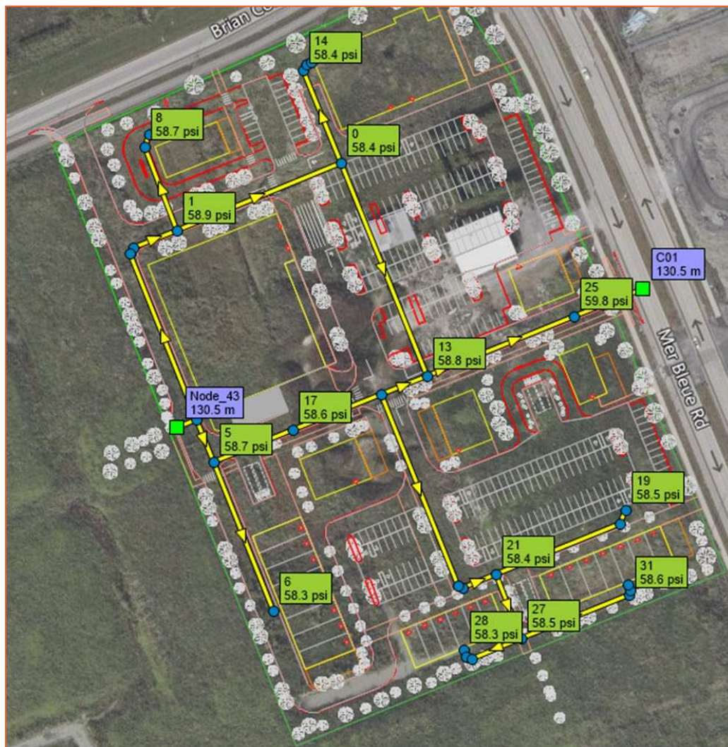
Figure 3.2: Maximum Pressures in the commercial block during AVDY Conditions
