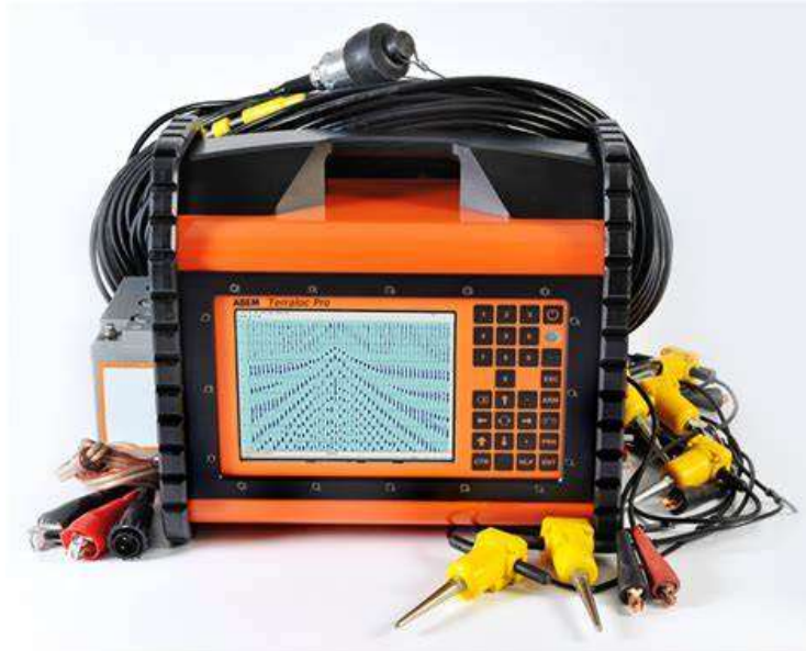
Figure 4: ABEM Terraloc Pro 2 – 24 Channel Seismograph with 4.5Hz geophones.
