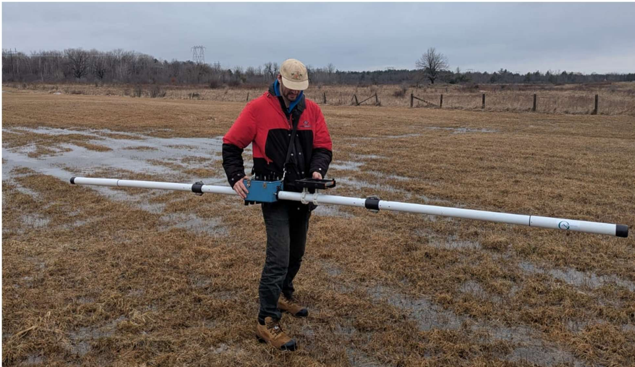
Figure 2: Geonics EM-31 Mk2 on site
