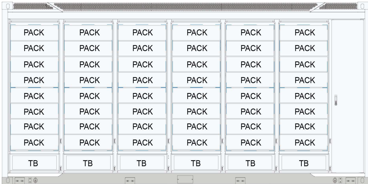
Figure 4 - Example Battery Stack Configuration
