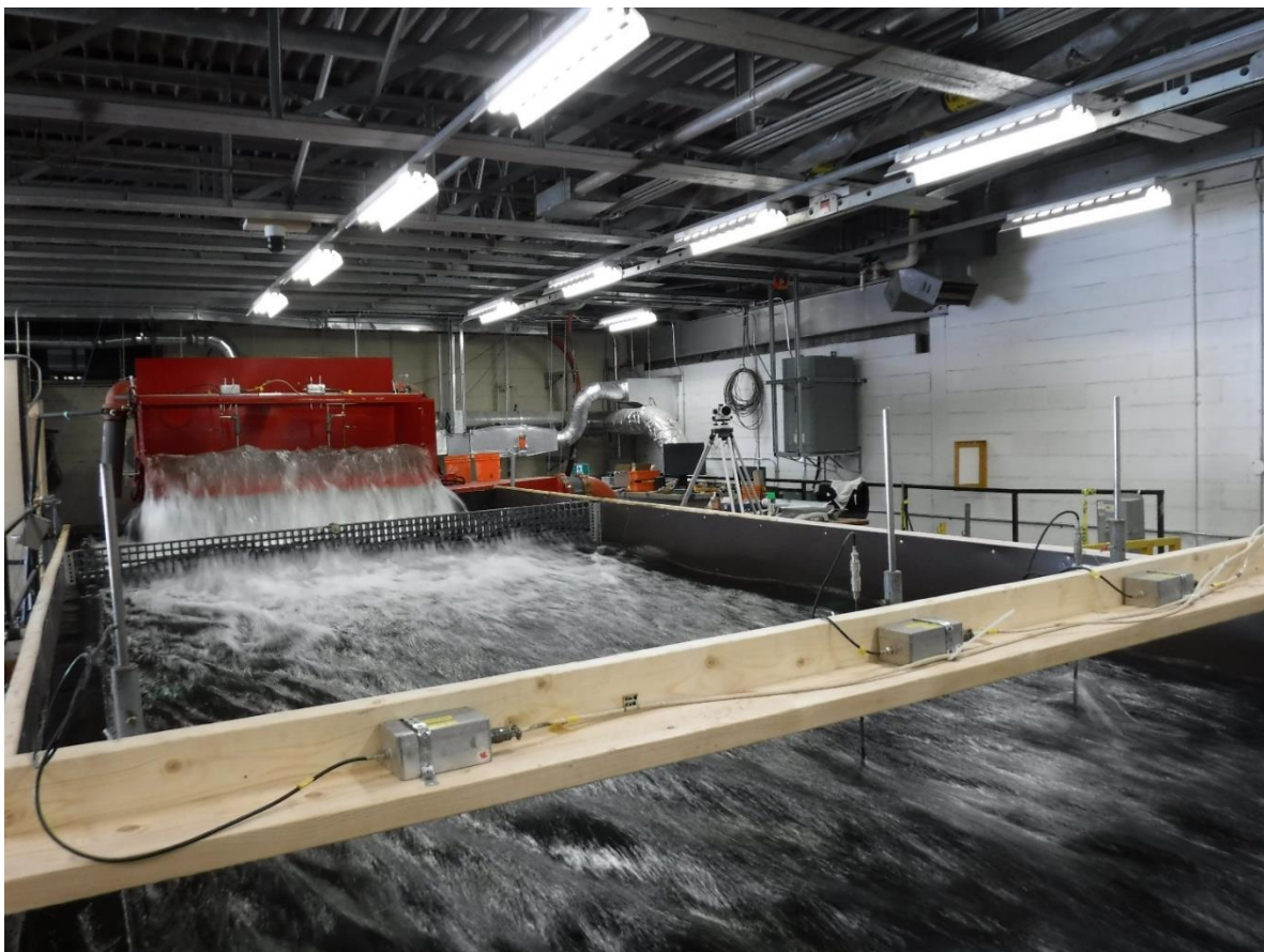
Figure 19. Water flowing from the head tank to the roadway during a high flow condition.
