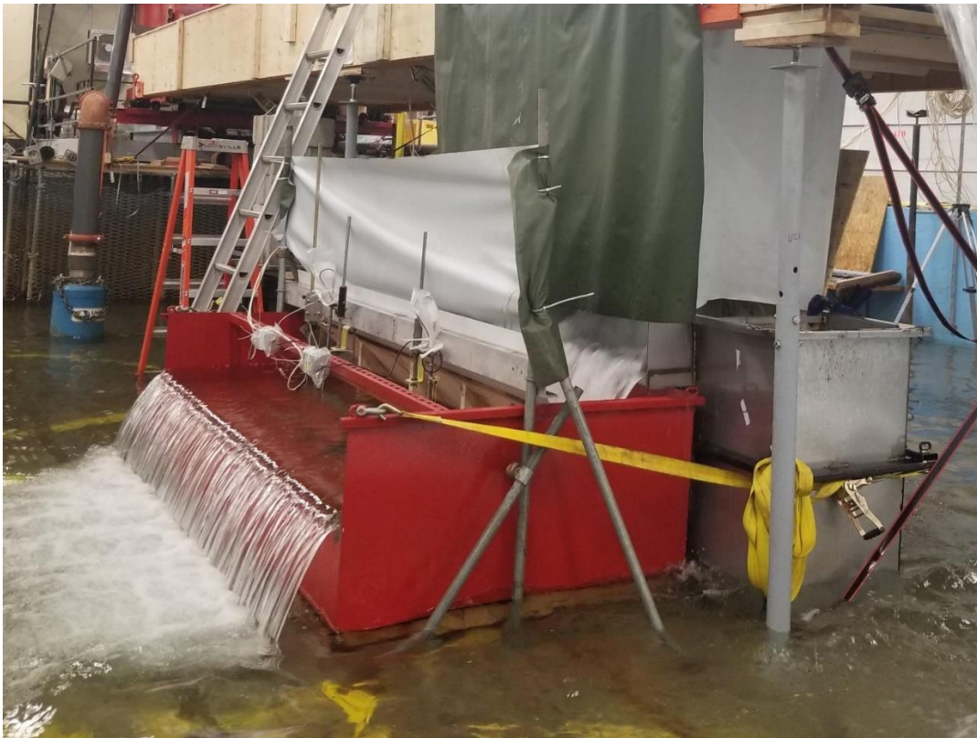
Figure 6. Photo of the settlement and measurement tanks that were used to capture the water that flowed through the catch basin inlet.
