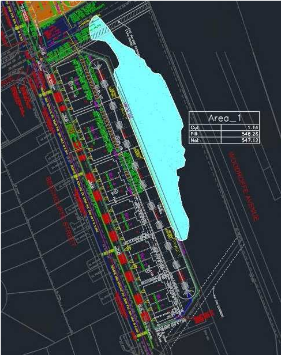
Figure 2 (Ultimate Condition): Quantifies the residual storage capacity (550 m 3 ) maintained at the toe of the slope outside of the proposed site plan limits, which acts in conjunction with the new SWMF. Volumes were calculated using the City of Ottawa 2024 DEM referenced to CGG2013a.
