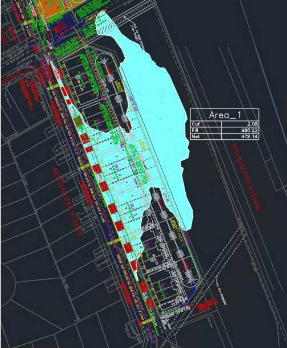
Figure 1 (Existing Condition): Analyzes topography on the subject property behind the curb line. Existing relief storage below the 88.05m spill elevation is approximately 980 m 3 . Volumes were derived using the City of Ottawa 2024 Digital Elevation Model (DEM) referenced to CGG2013a.
