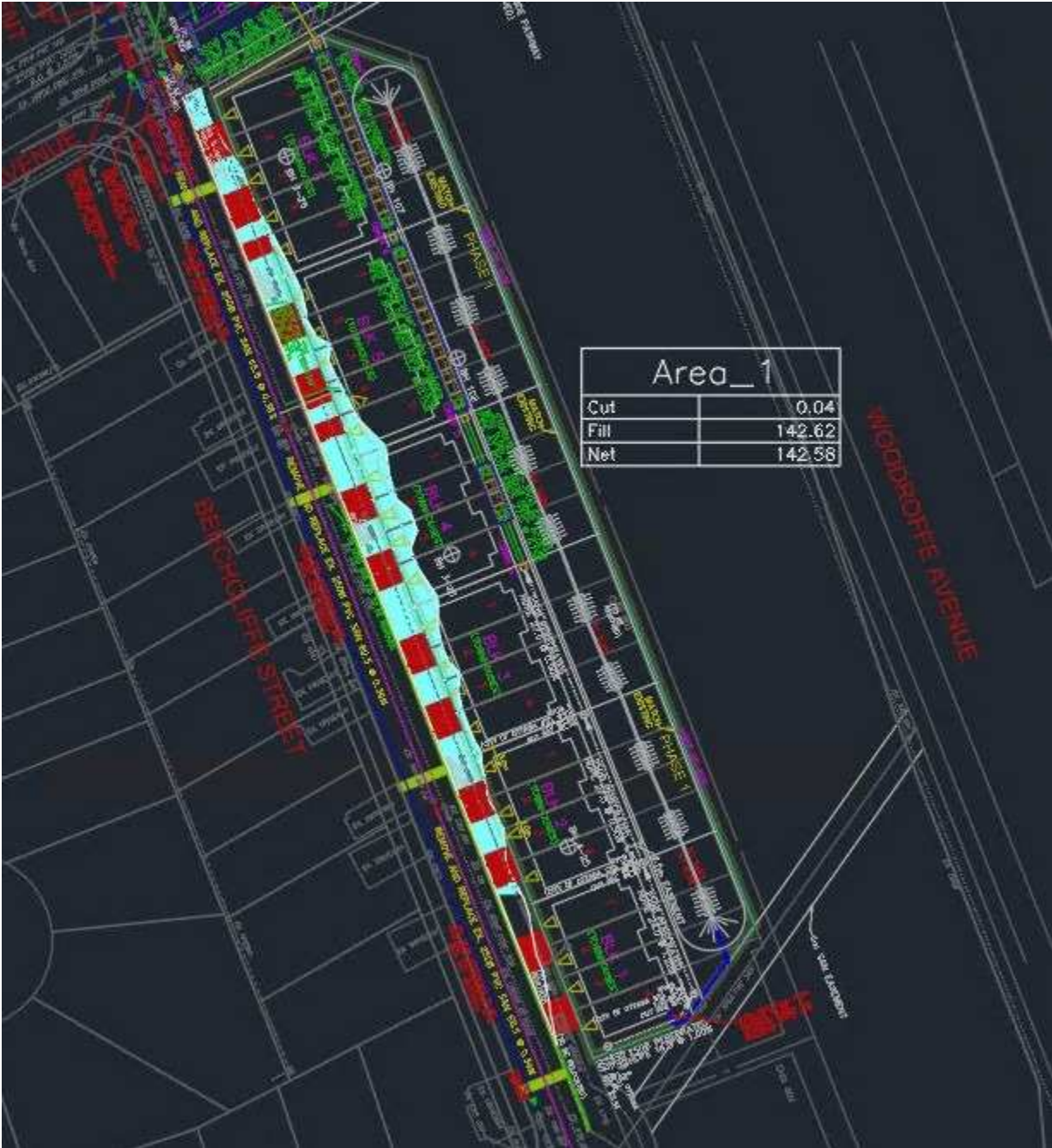
Figure 3 (Proposed Design): Evaluates the DSEL design against the adjusted spill elevation, providing 140 m 3 of storage. Volumes were calculated using DSEL design grades referenced to CGVD28 and spill elevation of 88.36 as discussed above.
