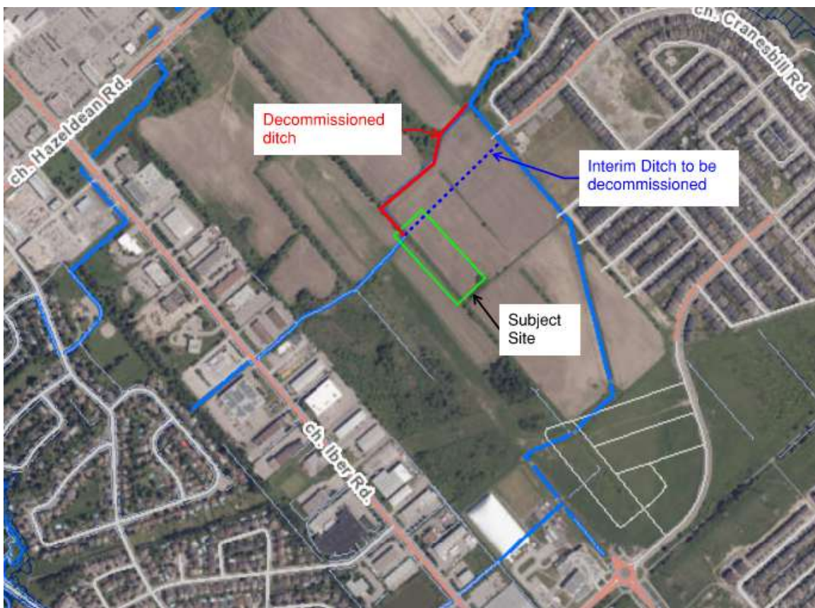
Figure 5.1 Existing Drainage Features
