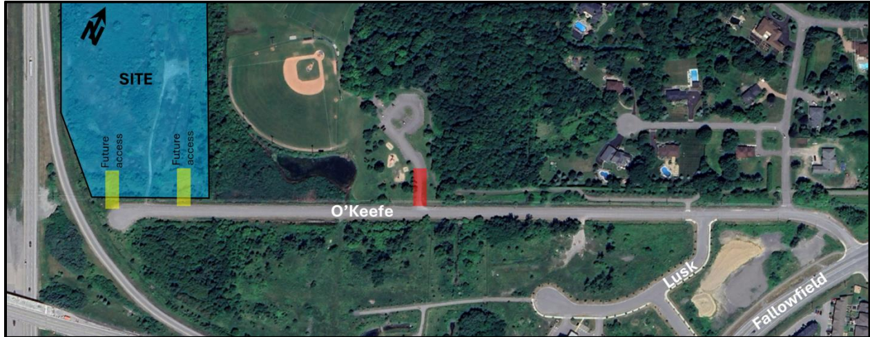
Figure 3: Adjacent Driveways within 200m of Site Access
