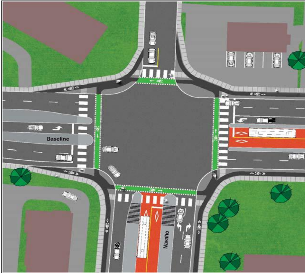
Figure 8: Protected Intersection Design
