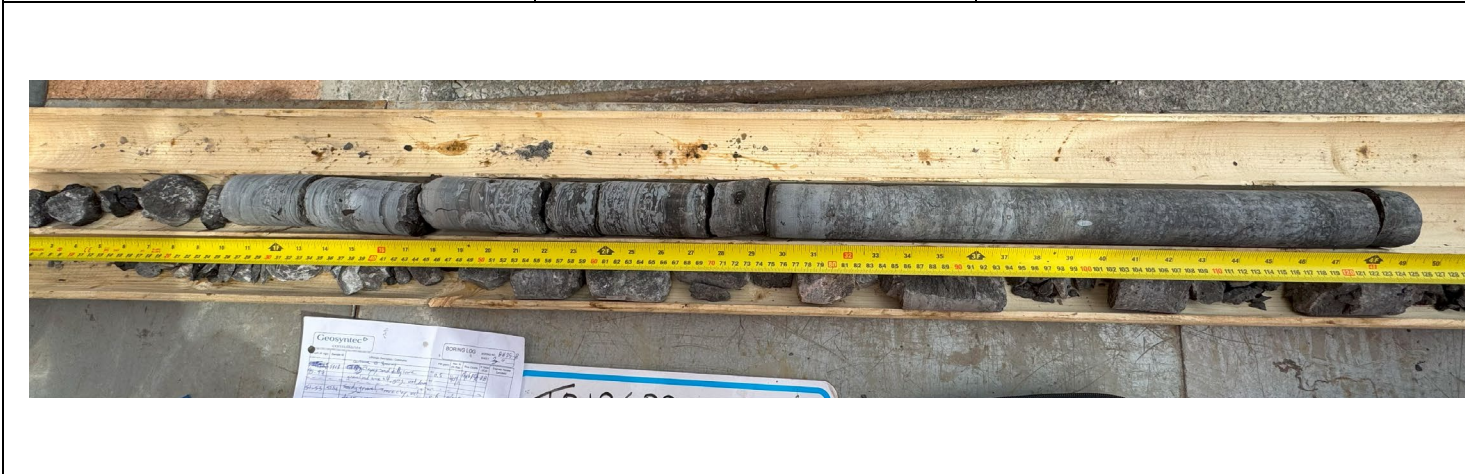
Borehole 25-08 Depth: 19.4 m – 20.6 m Bedrock, Run2, RQD 80%
