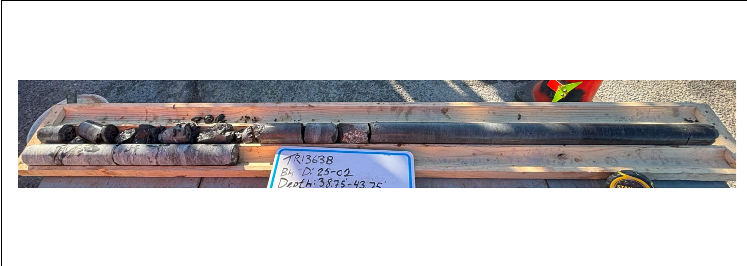
Borehole 25-02 Depth: 11.8 m – 13.3 m Bedrock, Run2, RQD 52%
