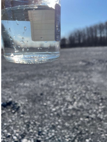
In-field observations of water during eight (8) hour pumping test. In-field turbidity measurement of 1.19 NTU after one (1) hour of pumping
