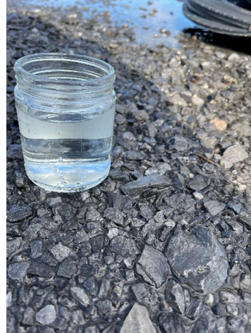
In-field observations of water during eight (8) hour pumping test. In-field turbidity measurement of 0.59 NTU after six (6) hour of pumping
