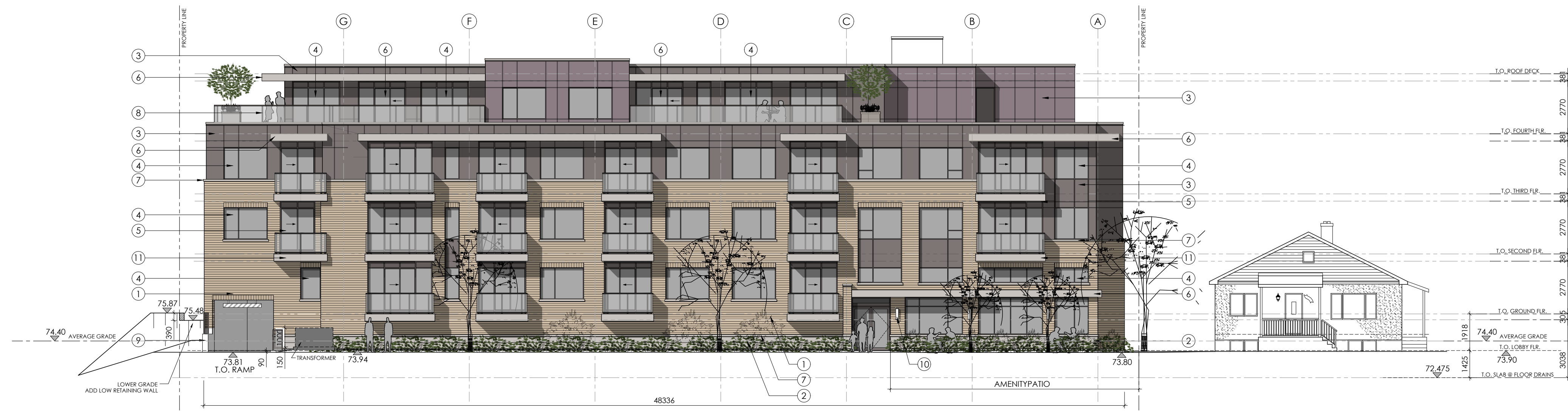
FRONT (NORTH) ELEVATION
