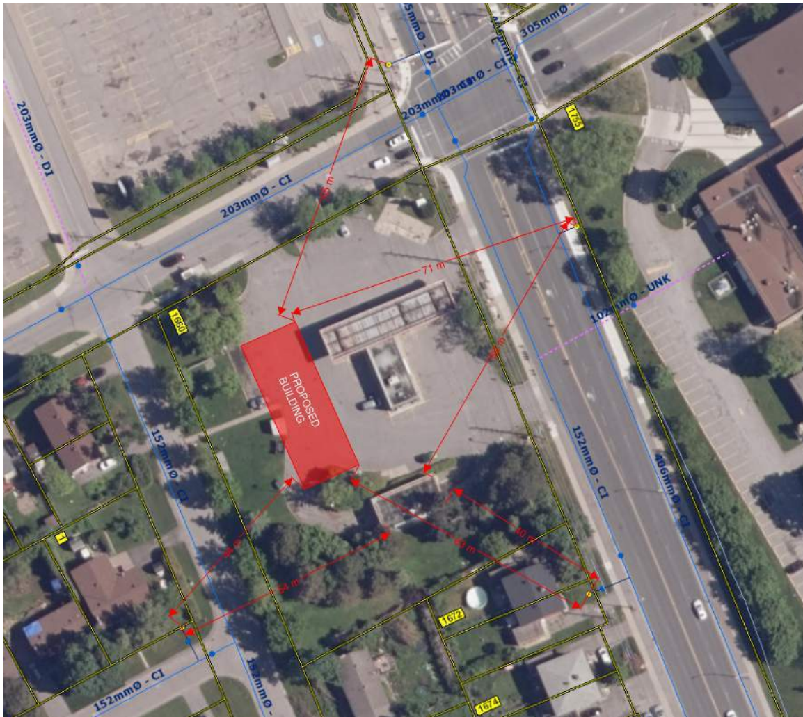
Figure 2 - Fire Hydrant Location
