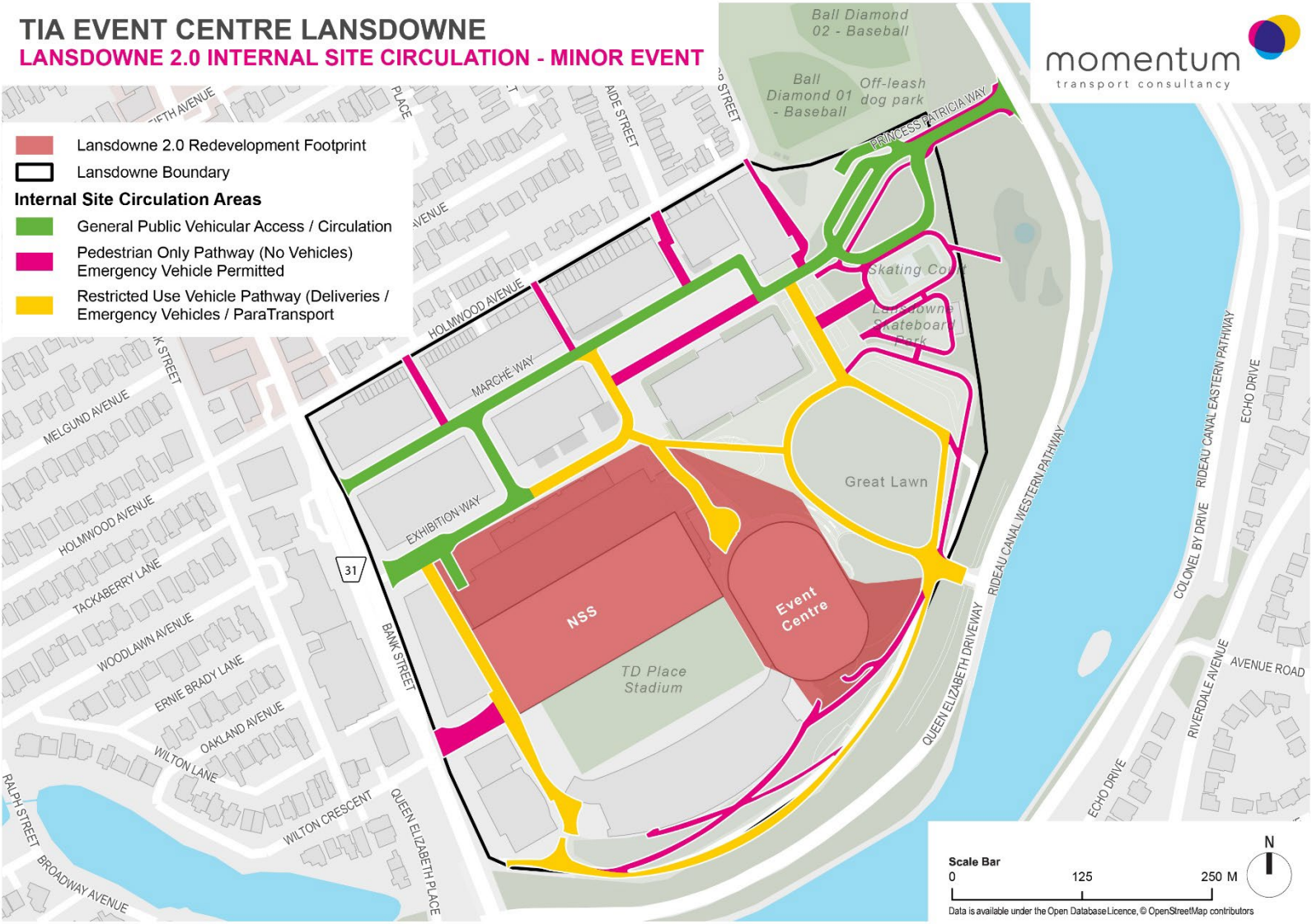
Figure 4.2: Lansdowne 2.0 Internal Site Circulation Plan (Minor Events)
