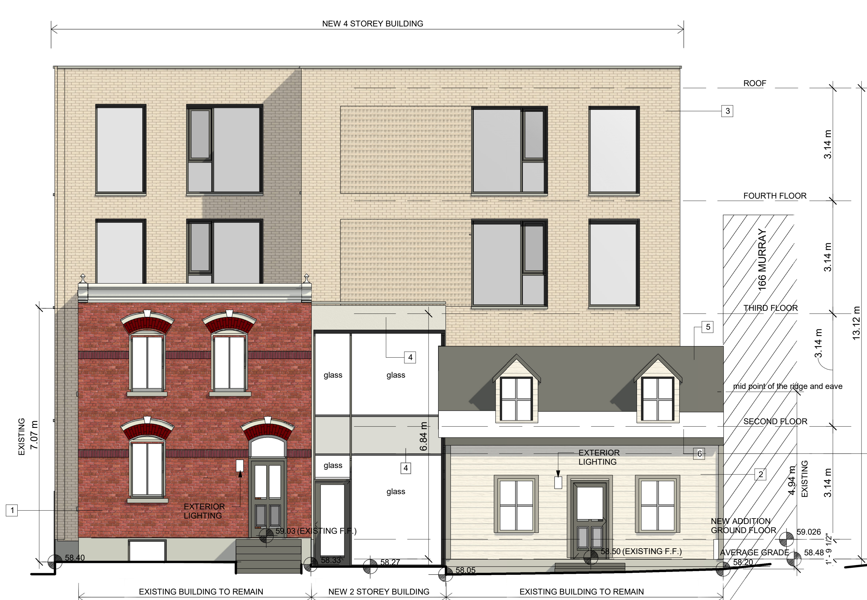
1 Front (North) Elevation 3/16" = 1'-0"
