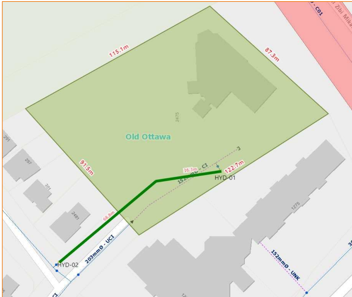
Figure 3.1: Existing Fire Hydrant Coverage Map
