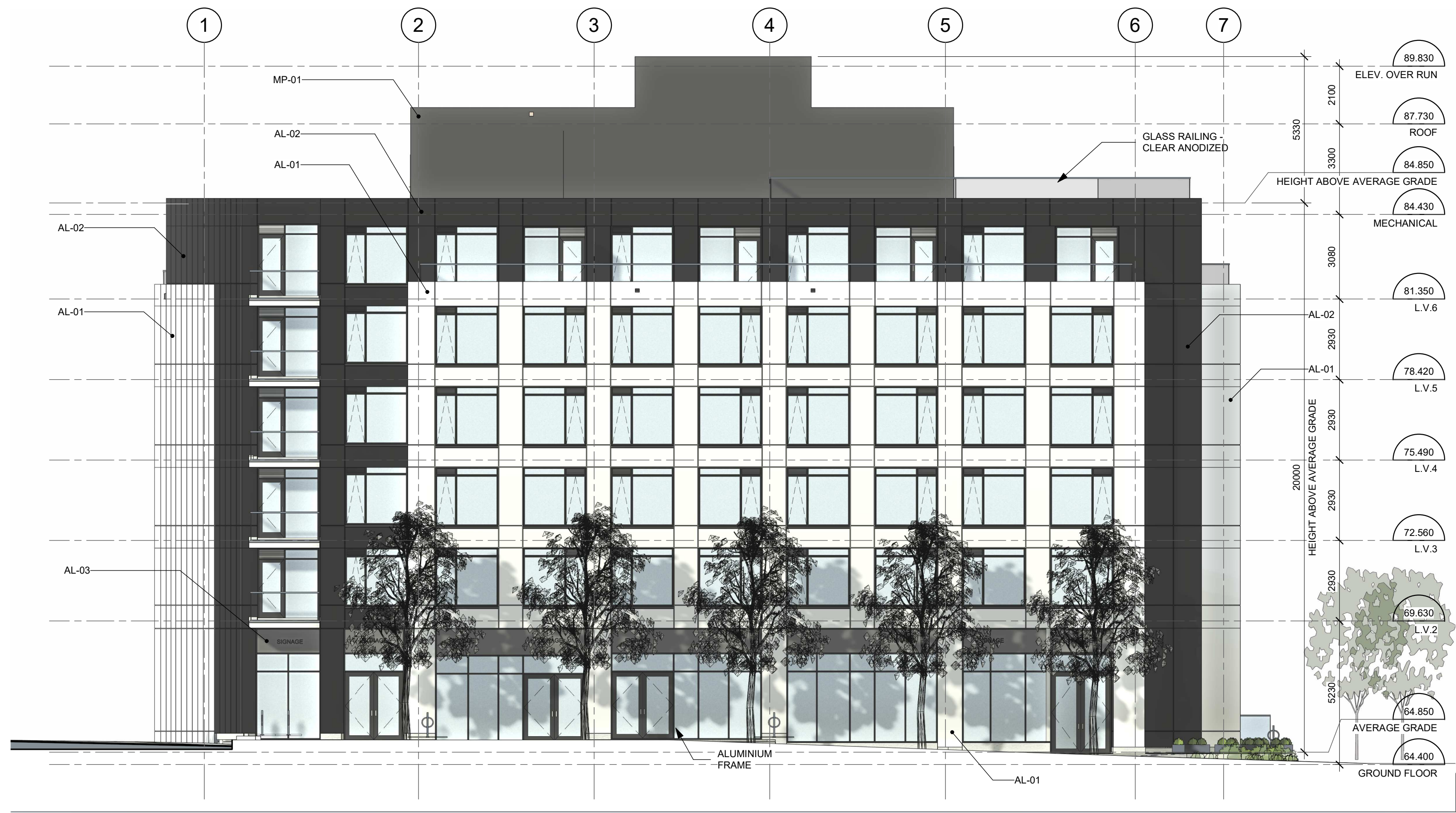
1 WEST ELEVATION - MAIN STREET D107 1:125
