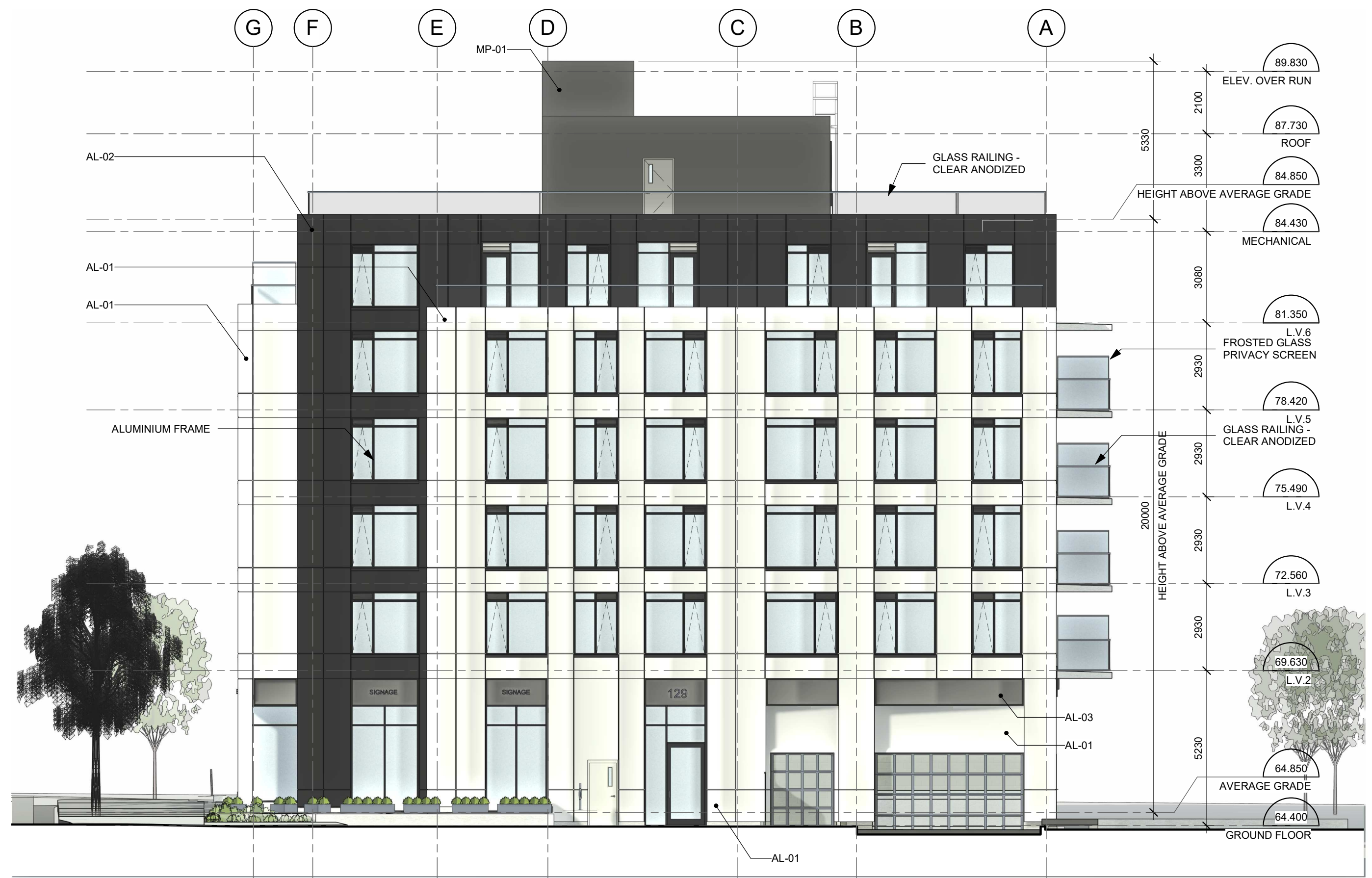
2 SOUTH ELEVATION - SPRINGHURST AVE D107 1:125
