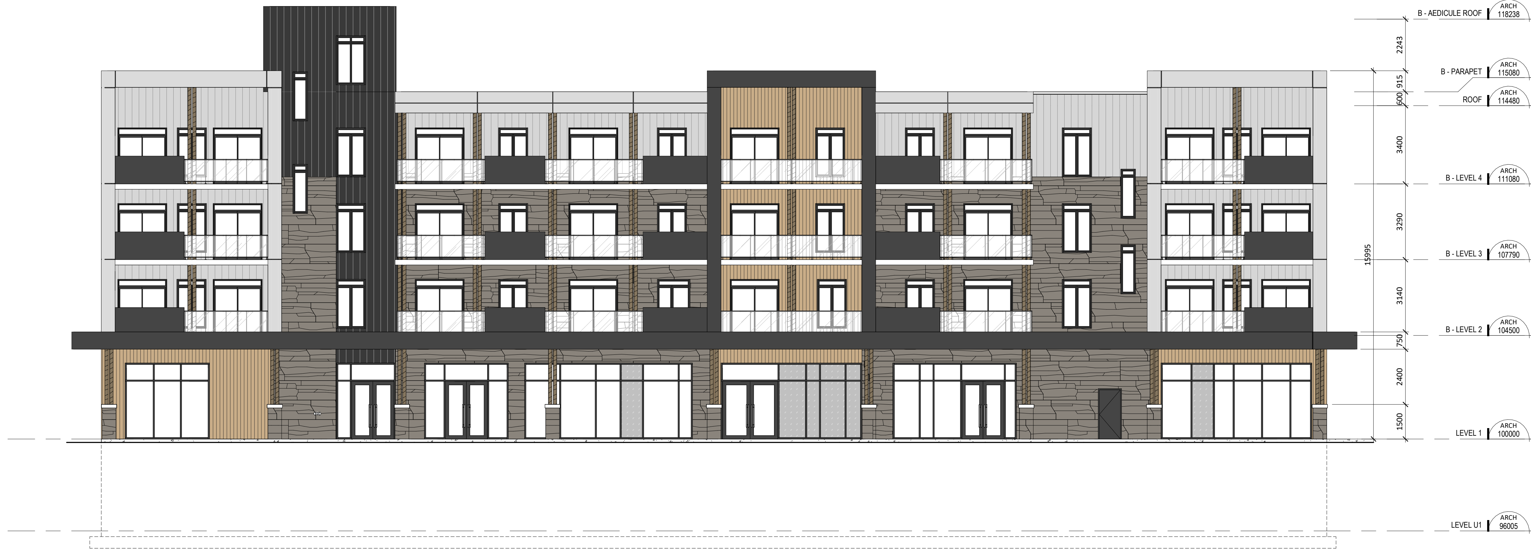
1 FRONT ELEVATION - BUILDING B A302 1:100
