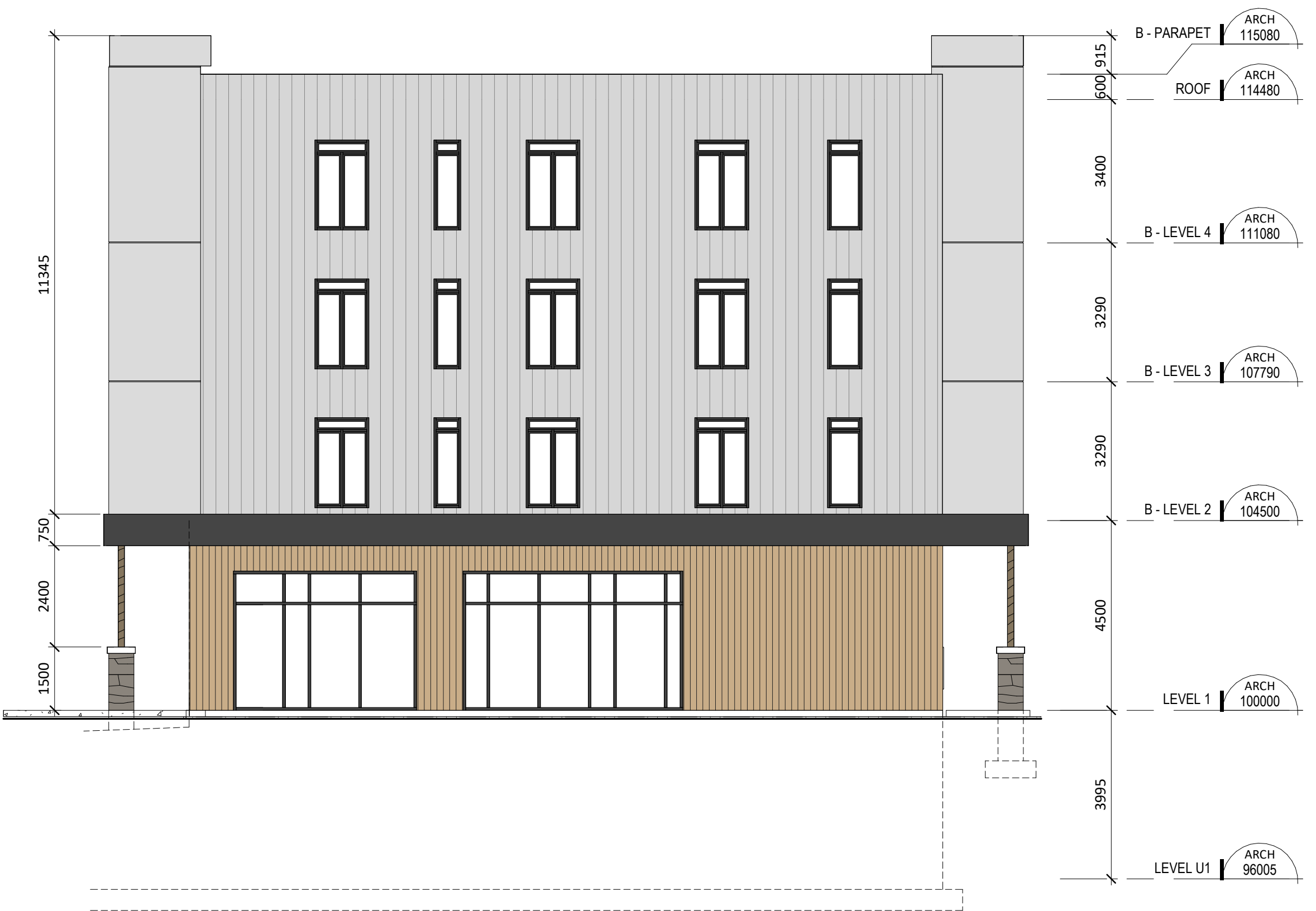
3 LEFT ELEVATION - BUILDING B A302 1:100
