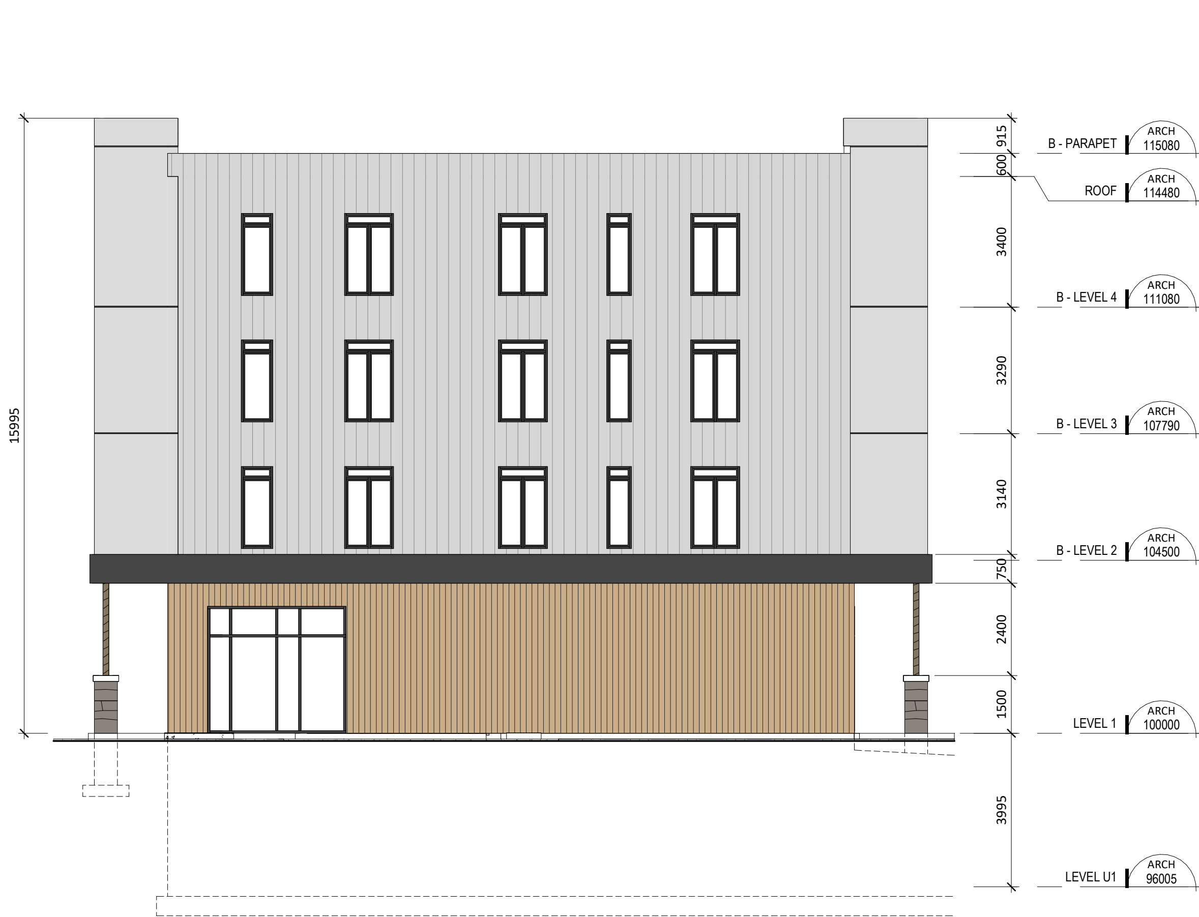
2 RIGHT ELEVATION - BUILDING B A302 1:100
