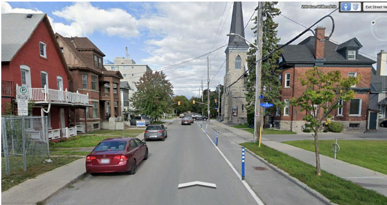
Figure 7: Street view looking east on Wilbrod from the development site. Note the two and three-storey detached residences generally clad in brick set on limestone foundations with varying roof forms and front porches. The building with the gable roof to the left is one of three buildings constructed in 1876 two of which will be demolished as part of the proposed development. Note the landscape character of the streetscape. Source: Google Earth.
