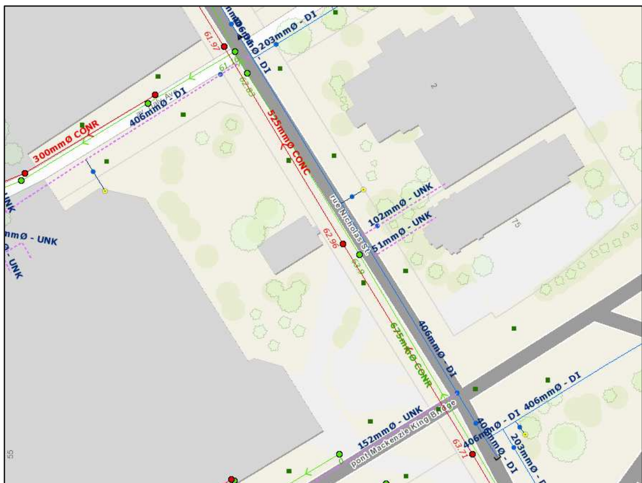
Figure 2: Existing Municipal Infrastructure Surrounding the Site
