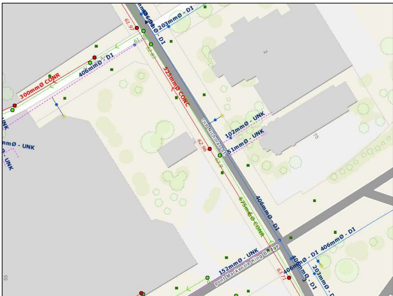
Figure 2: Existing Municipal Infrastructure Surrounding the Site
