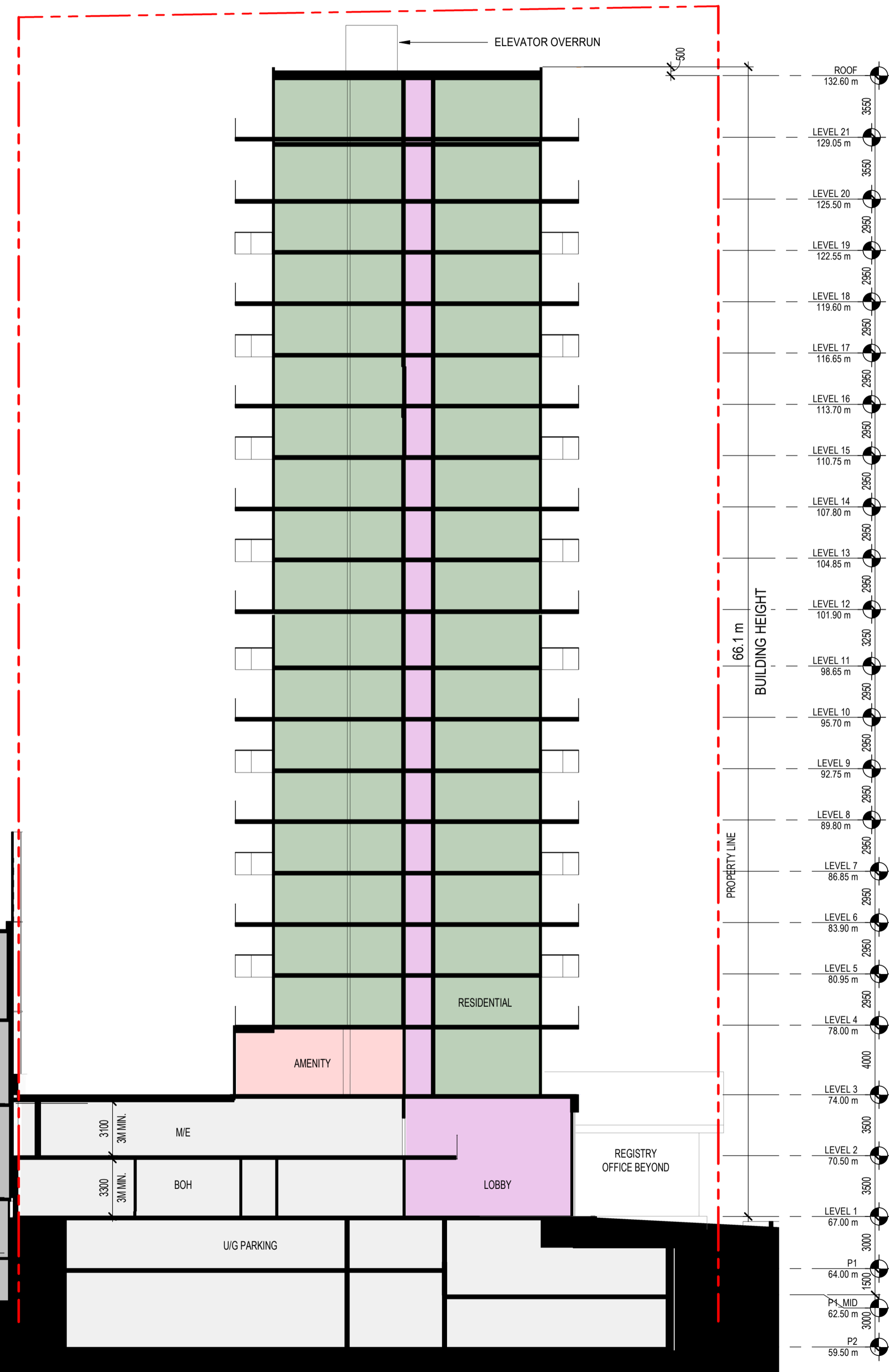
SOUTH TOWER SECTION THRU MAIN ENTRANCE
