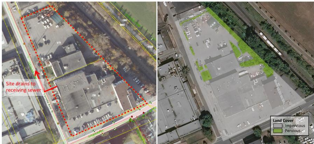
Figure 2: Existing Drainage (left) and Land Cover (right)
