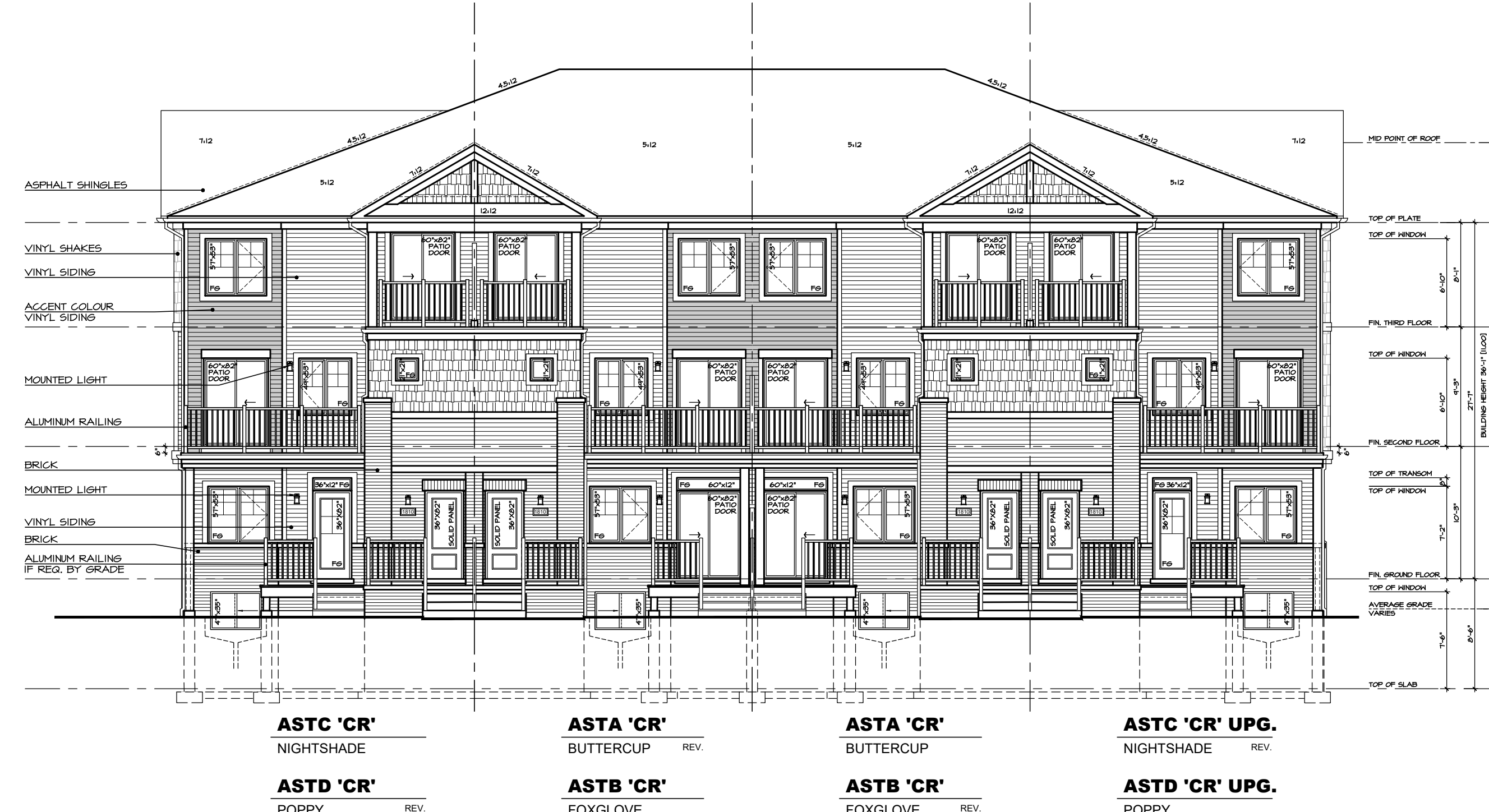
REAR ELEVATION - STREET SIDE
