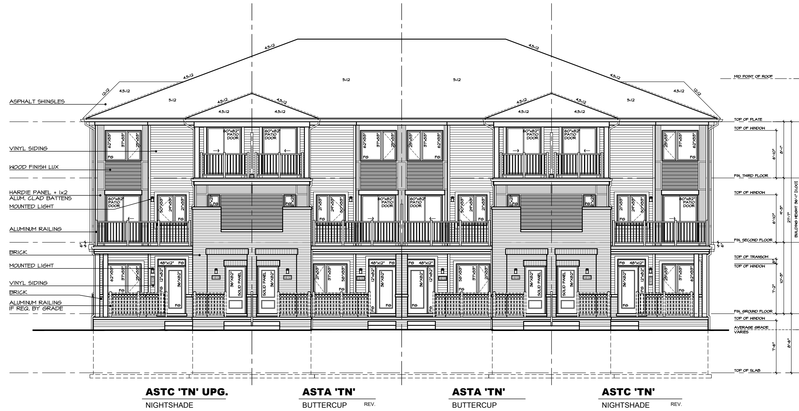
FRONT ELEVATION - SITE INTERIOR SIDE
